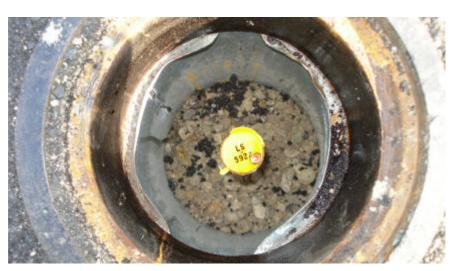
**OBSERVATION:** 3/4" IRON PIN WITH PLASTIC PLUG STAMPED LS 5922, IN MONUMENT BOX **MONUMENT REFERENCE:** 1/4 SECTION CORNER COMMON TO SECTIONS 19 & 30, T.1S., R.7E., M.D.B.&M.
