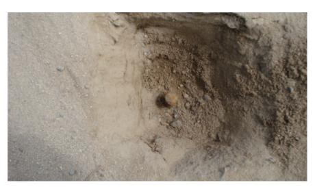
**OBSERVATION:** 1/2" IRON PIN (REBAR), NO TAG, 3" DOWN **MONUMENT REFERENCE:** 1/4 SECTION CORNER COMMON TO SECTIONS 34 & 35, T.1S., R.7E., M.D.B.&M.
