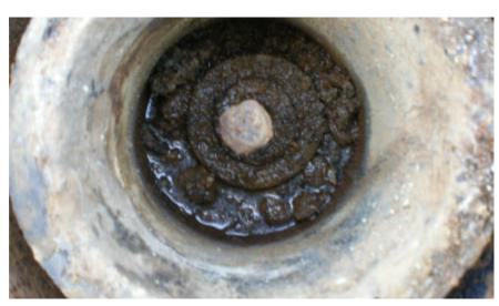
**OBSERVATION:** 1/2" SQUARE SPIKE WITH 2" WASHER IN MONUMENT BOX **MONUMENT REFERENCE:** 1/4 SECTION CORNER COMMON TO SECTION 36, T.1S., R.7E. & SECTION 31, T.1S.,
