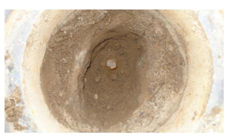
**OBSERVATION:** 1/2" IRON ROD IN MONUMENT BOX, NO TAG **MONUMENT REFERENCE:** 1/4 SECTION CORNER COMMON TO SECTION 32, T.1S. & SECTION 4, T.2S.,
