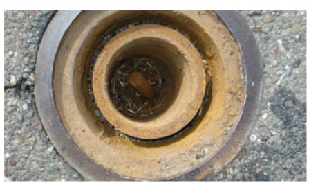
**OBSERVATION:** 3/4" IRON PIN (REBAR) IN MONUMENT BOX, NO TAG, BENT SOUTHEASTERLY **MONUMENT REFERENCE:** SECTION CORNER COMMON TO SECTIONS 25 & 36, T.1S., R.7E. & SECTIONS 30 & 31,
