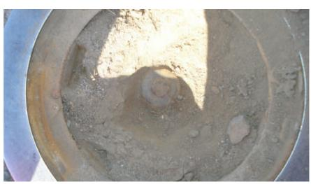
**OBSERVATION:** 2" BRASS WASHER STAMPED LS 2239 ON IRON PIN IN MONUMENT BOX **MONUMENT REFERENCE:** SECTION CORNER COMMON TO SECTION 36, T.1S., SECTION 1 T.2S., R.6E.,
