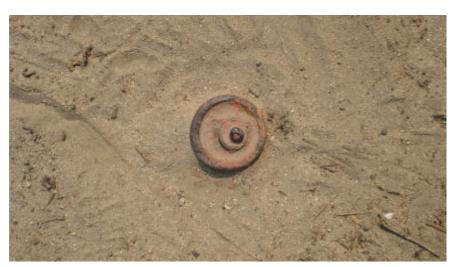
**OBSERVATION:** 1/2" IRON PIN IN 3/4" IRON PIPE WITHIN 2" IRON PIPE, NO TAG, AT SURFACE **MONUMENT REFERENCE:** 1/4 SECTION CORNER COMMON TO SECTIONS 35 & 36, T.1S., R.7E., M.D.B.&M.
