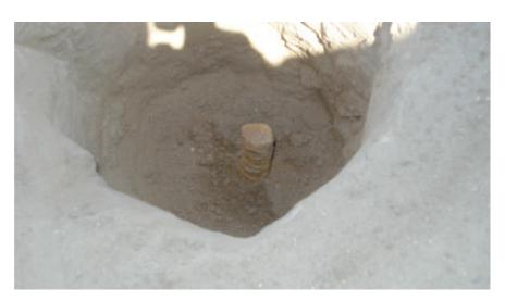
**OBSERVATION:** 3/4" IRON PIN (REBAR), NO TAG, 6" DOWN **MONUMENT REFERENCE:** CENTER OF SECTION 36, T.1S., R.7E., M.D.B.&M.
