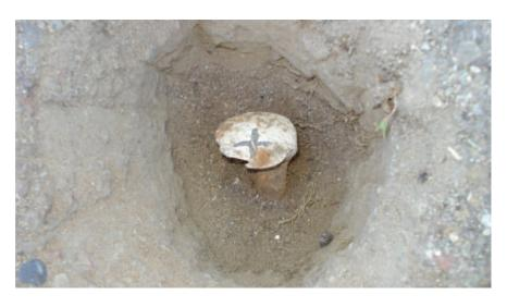
**OBSERVATION:** RAILROAD SPIKE IN PAVEMENT, BENT EASTERLY, 0.1' DOWN, NO TAG **MONUMENT REFERENCE:** 1/4 SECTION CORNER COMMON TO SECTIONS 30 & 31, T.1S., R.7E., M.D.B.&M.
