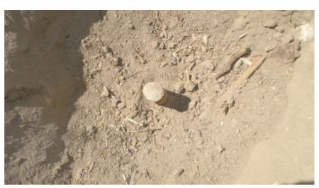
**OBSERVATION:** 3/4" IRON PIN (REBAR), NO TAG, 6" DOWN **MONUMENT REFERENCE:** CENTER OF SECTION 36, T.1S., R.6E., M.D.B.&M.
