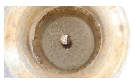
**OBSERVATION:** 3/4" IRON PIN (REBAR) IN MONUMENT BOX, NO TAG **MONUMENT REFERENCE:** 1/4 SECTION CORNER COMMON TO SECTION 24, T.1S., R.7E. & SECTIONS 19, T.1S.,
