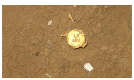
OBSERVATION: 3/4" IRON PIPE WITH PLASTIC PLUG STAMPED LS 6406, DOWN 1/5'
