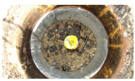
**OBSERVATION:** 3/4" IRON PIPE WITH PLASTIC CAP STAMPED LS 5922 IN MONUMENT BOX **MONUMENT REFERENCE:** 1/4 SECTION CORNER COMMON TO SECTION 24, T.1S., R.6E. & SECTION 19,
