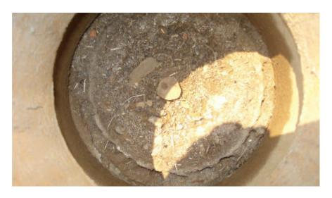
**OBSERVATION:** 3/4" IRON PIN (REBAR) IN MONUMENT BOX, NO TAG **MONUMENT REFERENCE**: CENTER OF SECTION OF SECTION 33, T.1S., R.7E., M.D.B.&M. RECORDED REFERENCE: RS 33-133 (POINT NO. 248) (5/8" REBAR IN MON. WELL)
