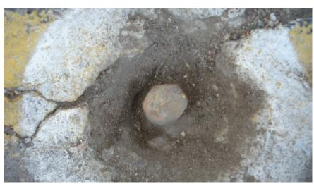
**OBSERVATION:** RAILROAD SPIKE IN PAEMENT, 0.1' DOWN, NO TAG **MONUMENT REFERENCE:** 1/4 SECTION CORNER COMMON TO SECTIONS 25 & 36, T.1S., R.6E., M.D.B.&M.
