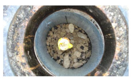
OBSERVATION: 3/4" IRON PIPE WITH PLASTIC CAP STAMPED LS 5922 IN MONUMENT BOX MONUMENT REFERENCE: 1/4 SECTION CORNER COMMON TO SECTIONS 19 & 20, T.1S., R.7E., M.D.B.&M.
