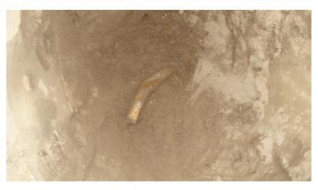
**OBSERVATION:** 3/4" IRON PIN, TAGGED R.C.E. 8189, BENT SOUTHEASTERLY, 1.2' DOWN **MONUMENT REFERENCE**: CENTER OF SECTION 25, T.1S., R.7E., M.D.B.&M.
