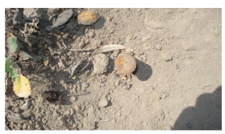
**OBSERVATION:** 3/4" IRON PIN, NO TAG, EXTENDING ABOVE GRADE **MONUMENT REFERENCE:** 1/4 SECTION CORNER COMMON TO SECTIONS 25 & 26, T.1S., R.7E., M.D.B.&M.
