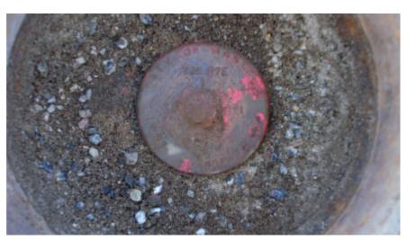
**OBSERVATION:** 2 1/2" BRASS DISK STAMPED CITY OF MANTECA RCE 18420 ON IRON PIN IN MONUMENT.BOX **MONUMENT REFERENCE:** 1/4 SECTION CORNER COMMON TO SECTIONS 20 & 21, T.1S., R.7E., M.D.B.&M.
