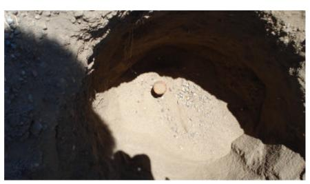
**OBSERVATION:** 3/4" IRON PIPE, 1.2' DOWN, NO TAG **MONUMENT REFERENCE:** 1/4 SECTION CORNER COMMON TO SECTIONS 13 & 24, T.2S., R.6E., M.D.B.&M.
