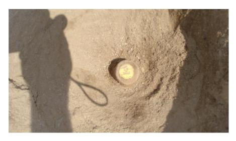
**OBSERVATION:** 1 1/4" IRON PIPE WITH PLASTIC PLUG STAMPED LS 5443, 1.6' DOWN **MONUMENT REFERENCE**: CENTER OF SECTION 12, T.2S., R.7E., M.D.B.&M.
