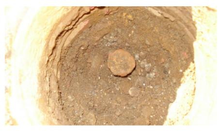
**OBSERVATION:** 1" IRON PIN (REBAR), NO TAG, IN MONUMENT BOX **MONUMENT REFERENCE:** SECTION CORNER COMMON TO SECTIONS 7, 8, 17 & 18, T.2S., R.7E., M.D.B.&M.
