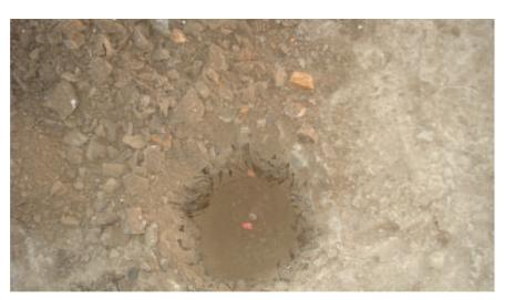
OBSERVATION: 3/4" IRON PIN (REBAR), 0.8' DOWN, NO TAG MONUMENT REFERENCE: 1/4 CORNER COMMON TO SECTIONS 14 & 15, T.2S., R.6E., M.D.B.&M.
