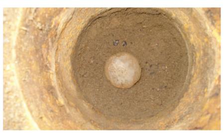
**OBSERVATION:** 2" BRASS DISK, STAMPED RE 9338 IN MONUMENT BOX, BOX 0.7' DOWN **MONUMENT REFERENCE:** 1/4 SECTION CORNER COMMON TO SECTIONS 8 & 17, T.2S., R.7E., M.D.B.&M.
