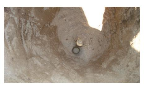
**OBSERVATION:** 3/4" IRON PIPE WITH PLASTIC CAP STAMPED LS 5443, 1.5' DOWN
