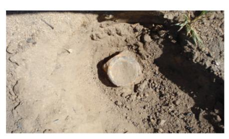
**OBSERVATION:** 2" IRON PIPE, 0.3' DOWN, NO TAG, AT BASE OF SOUTH FACE OF POST
