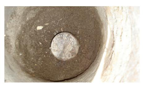
**OBSERVATION:** 2" BRASS DISK, STAMPED RE 9338, ON IRON PIN IN MONUMENT BOX **MONUMENT REFERENCE:** SECTION CORNER COMMON TO SECTIONS 22, 23, 26 & 27, T.2S., R.7E., M.D.B.&M.
