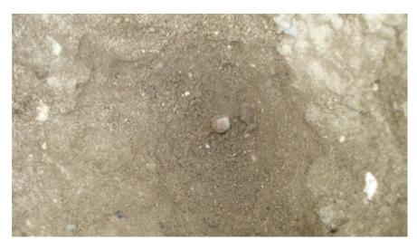
**OBSERVATION:** 1/2" IRON PIN (REBAR), 1.0' DOWN, NO TAG **MONUMENT REFERENCE:** 1/4 SECTION CORNER COMMON TO SECTIONS 16 & 21, T.2S., R.7E., M.D.B.&M.
