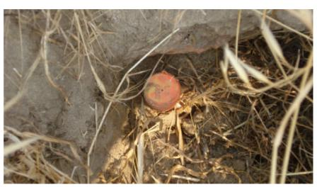
OBSERVATION: 3/4" IRON PIPE WITH PLASTIC CAP STAMPED L.S. 4450, 0.8' DOWN
