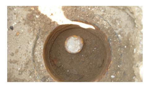
**OBSERVATION:** 2" BRASS DISK, NO MARKINGS, IN MONUMENT BOX, BOX 0.7' DOWN **MONUMENT REFERENCE:** 1/4 SECTION CORNER COMMON TO SECTIONS 17 & 20, T.2S., R.7E., M.D.B.&M.
