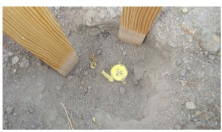
OBSERVATION: 3/4" IRON PIPE WITH PLASTIC CAP STAMPED LS 7126, 0.2' DOWN
