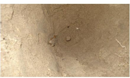
**OBSERVATION:** 5/8" IRON PIN (REBAR), 1.3' DOWN
