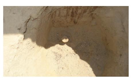
OBSERVATION: 1" IRON PIPE, 1.1' DOWN, NO TAG, AT BASE OF WEST FACE OF POST (RAILROAD TIE)
