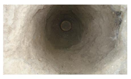
**OBSERVATION:** 2" IRON PIPE, 1.5' DOWN, NO TAG **MONUMENT REFERENCE**: CENTER OF SECTION 21, T.2S., R.7E., M.D.B.&M.
