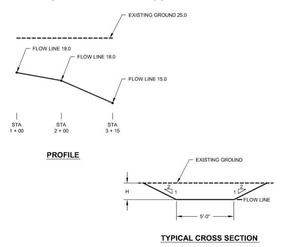
A farmer is excavating a ditch to drain an existing field. Using the given profile and typical cross section, calculate the quantity of excavated material.
