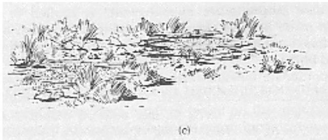
Corner monuments of the public land surveys. Reading from top of page: (a) Modern iron post with brass cap, and mound of stone; (b) wooden posts, the one on left not much more than a twig; (c) wooden post, showing decay at ground line; (d) corner monument obliterated, remnants of stone mounds identify corner position; (e) corner monument obliterated, evidence of old pits fixes corner position.
