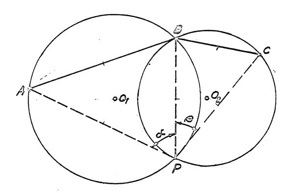
Sighting fixed points A, B, and E from an unknown position P, angles E and E are observed.
