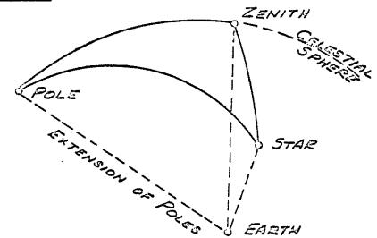
In the spherical triangle in the celestial sphere as chose above "P" represents the extension of the earth's pole, "Z" the observer's senith, and "S" the star being observed (sun or polaris). In the celestial triangle (P, Z, and S) there are six parts to the triangle (3 angles and 3 sides).
