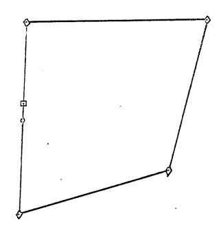
In retracing the exterior boundaries of a regular interior section (80 chains record length of each side) in preparation for subdivision of the section, all four original section corners were found. The west quarter corner was found on line between the NV and SV corners, but 500 feet north of its theoretical position. No other quarter corners were found.
